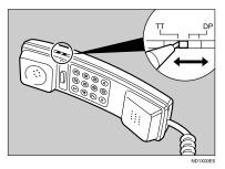
The switch on the handset should be in the appropriate position-TT (Tone Dialing) or DP (Pulse Dialing). Adjusting the handset bell volume
